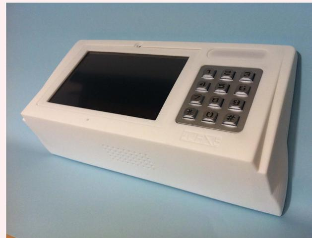
The next step will be to use the prototype to find out how it will comply with new Swedish regulations in official buildings. There are new rules of Duplex Communication with Quittance Possibilities at Temporary Evacuation Places. This new access card reader will be equipped with duplex video and voice and also some other functions to increase the demands.
