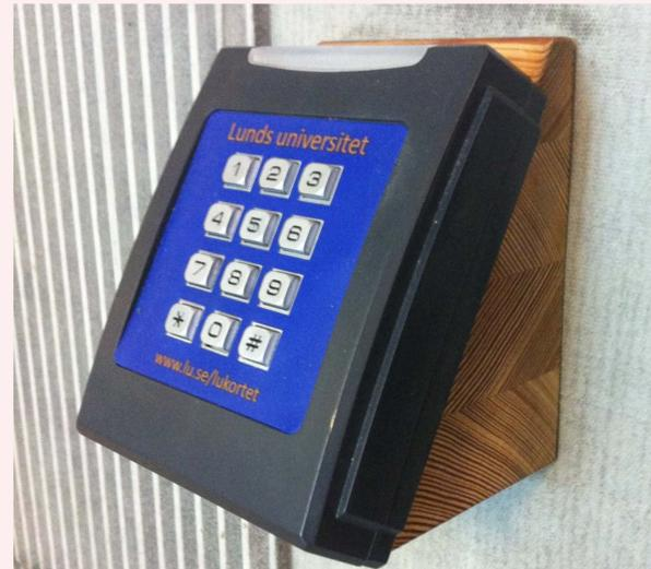
With the goal optimizing usability level we produced some test installations. The first solution was to cut pieces of wood, or plastic, at an angle that allowed us to install the readers at an angle that made the keypads more visible from a number of angles. Metal frames were also found to be not so good, because of interference problems with the magnet field used by RFID-systems. To solve this interference, there must be at least 25 mm of plastic between the card reader and the metal frame.
